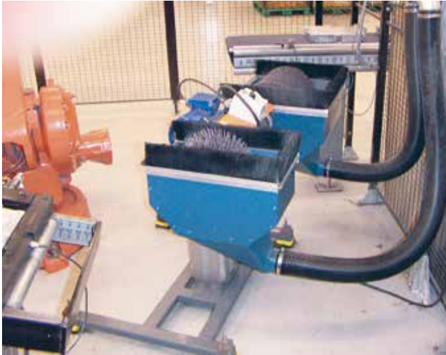
Robot deburring for telecom parts
