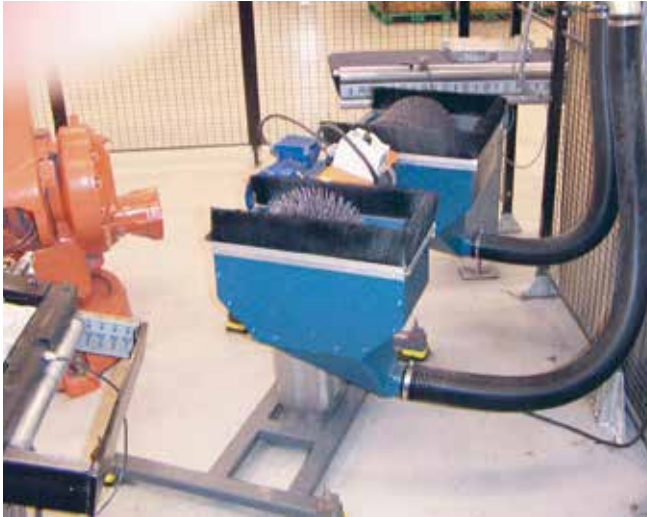
Robot deburring for telecom parts
