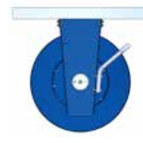
Hose guide installed upwards.
