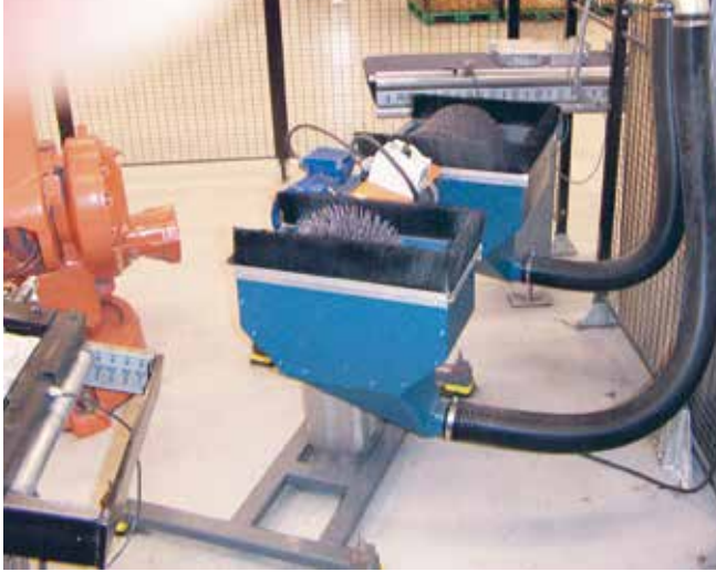
Robot deburring for telecom parts
